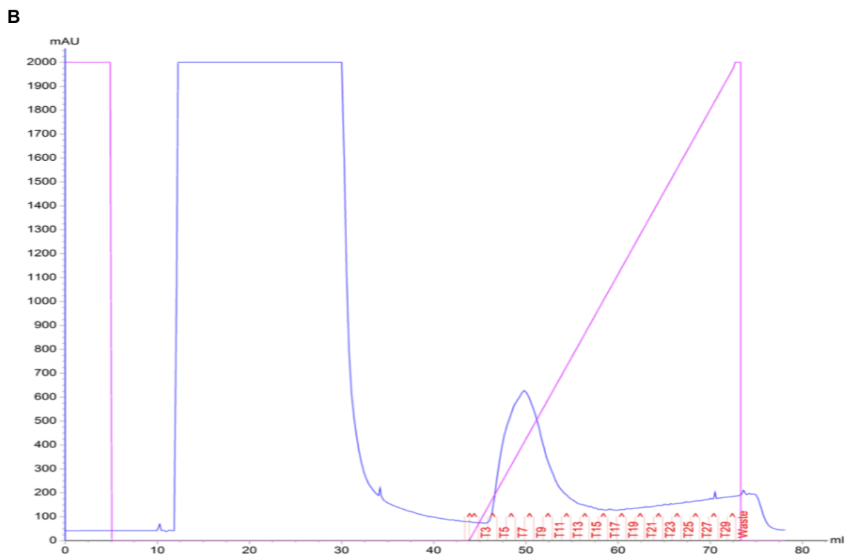
Figure 19 – Purification of His-tagged OmpR and FixJ proteins. Spectrum obtained by the ÄKTA system with automatic increase of imidazole. (A) shows the elution of OmpR protein and (B) shows FixJ.
